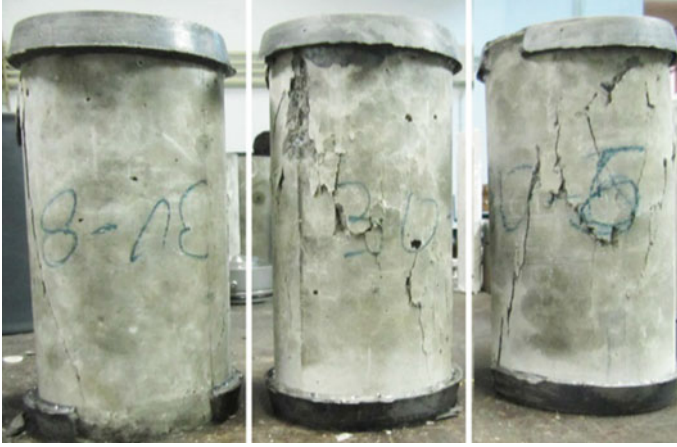
Fig. 4.13 RAC30%: failure modes in uniaxial compression
