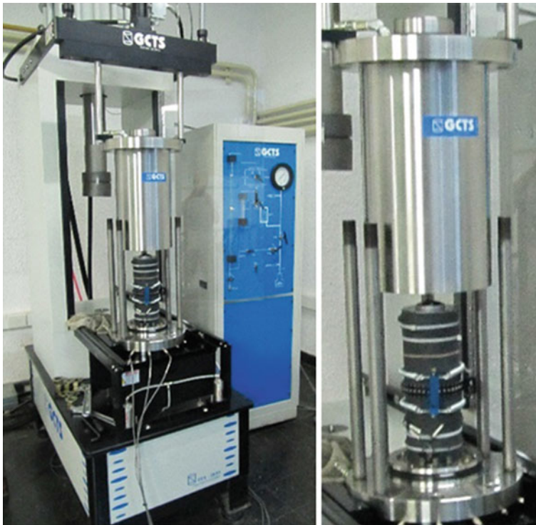
Fig. 4.8 General view of the GCTS compression frame (left) and the confining cell (right)
