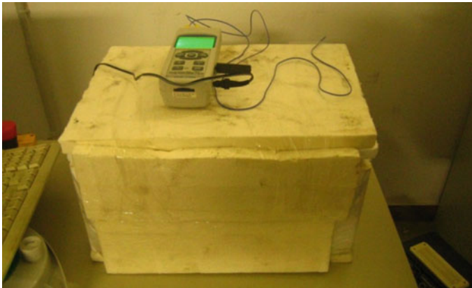
Fig. 2.5 Temperature measurement inside insulated mould
