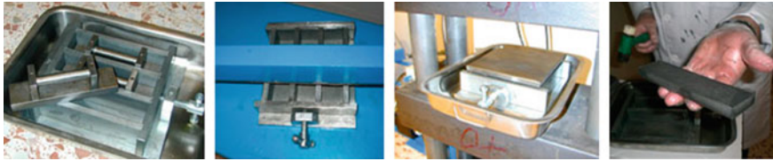
Fig. 9.16 Process employed by Claramunt et al. (2011a, b): mold and press system used to prepare the specimens (from left to right molds, vibrating table, pressing system and demolding)
