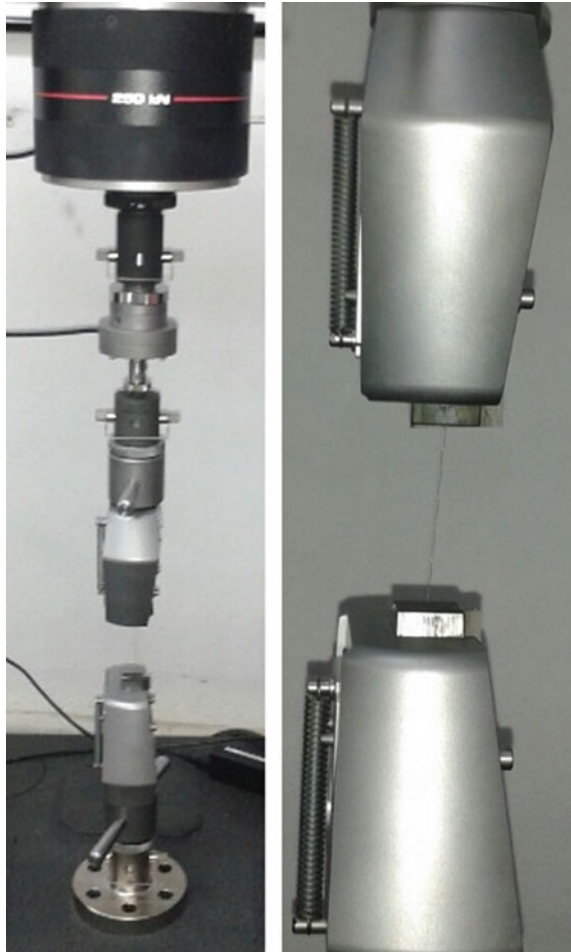
Fig. 8.9 Direct tensile test on recycled fibres. Photo credits Laboratory of Materials and Structures, University of Buenos Aires, 2014
