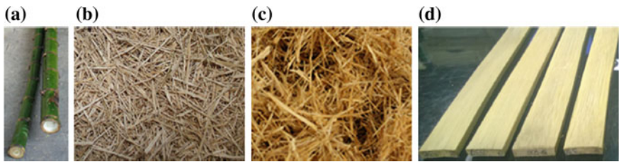
Fig. 9.117 Bamboo culms (a), air dried bamboo fibres (b), washed bamboo fibres before use if geopolymer composites (c) and reinforcing bamboo strips (d) (Sà Ribeiro et al. 2016)
