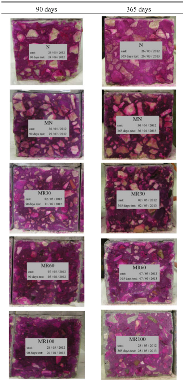
Fig. 3.24 Natural carbonation at 90 and 365 days of concrete samples containing medium amounts of FA
