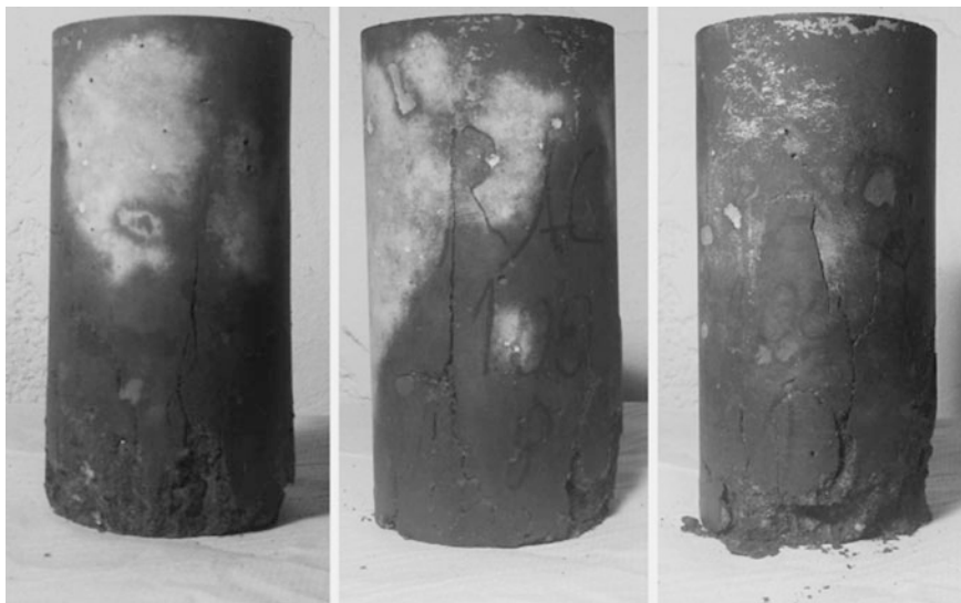
Fig. 4.27 RAC100%: failure modes in tri-axial compression for 4.5 MPa ( left ), 15 MPa ( center ) and 21 MPa ( right ) confinement levels
