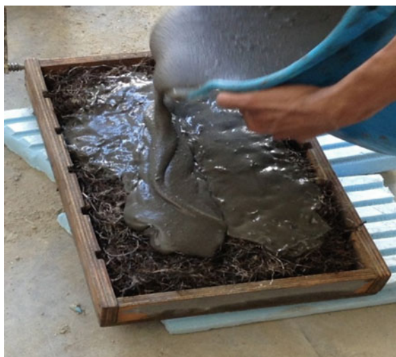
Fig. 8.19 Process of preparing RSFRC (Zamanzadeh 2017)
