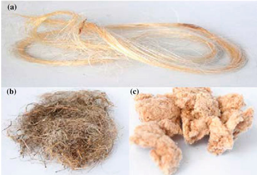
Fig. 9.1 Images of natural fibres in different forms: a strands, b staple, c pulp
