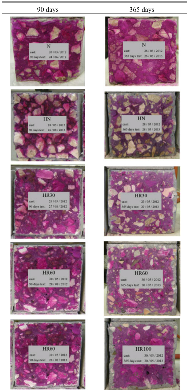
Fig. 3.25 Natural carbonation at 90 and 365 days of concrete samples containing highest amounts of FA
