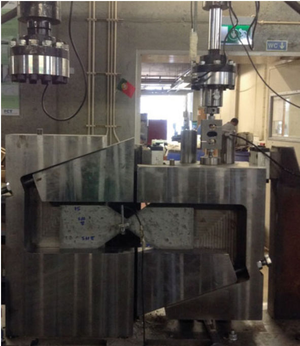
Fig. 11.8 Iosipescu test setup (Baghi and Barros 2016)
