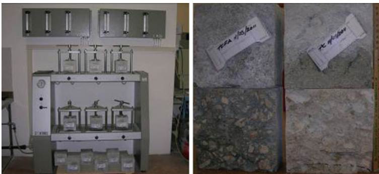
Fig. 3.16 Some concrete specimens during and after the permeability tests
