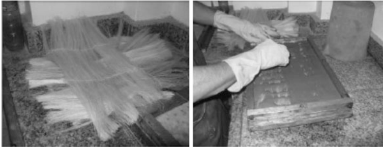
Fig. 9.100 Curaua fibre tissue and production of the laminates (from D’Almeida et al. 2009)
