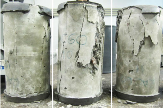
Fig. 4.14 RAC60%: failure modes in uniaxial compression
