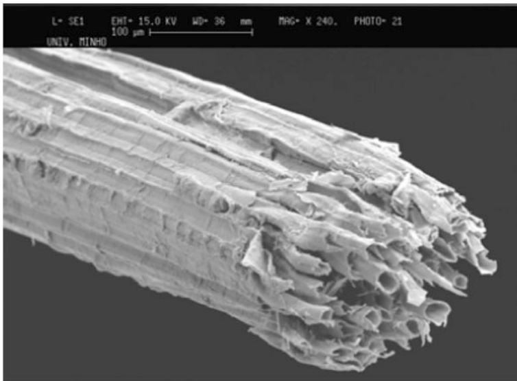
Fig. 9.105 Micrograph of fractured banana fibre (from Mukhopadhyay et al. 2008)
