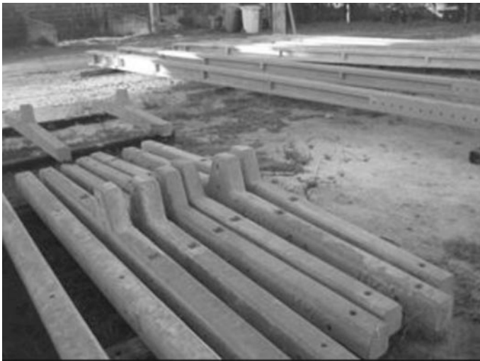
Fig. 13.15 Column type elements in concrete reinforced with vegetable fibres (Bragança et al. 2014)
