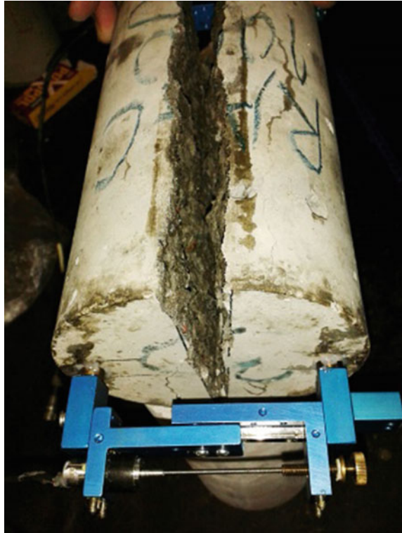
Fig. 4.15 Splitting tensile test: typical failure mode
