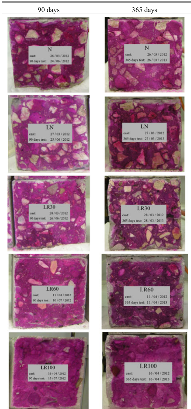
Fig. 3.23 Natural carbonation at 90 and 365 days of concrete samples containing low amounts of FA
