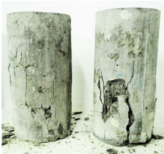
Fig. 4.26 RAC60%: failure modes in tri-axial compression for 4.5 MPa ( left ) and 15 MPa ( right ) confinement levels
