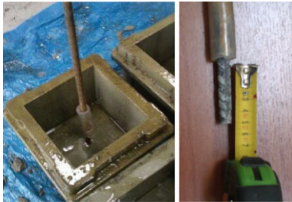
Fig. 3.6 Casting of samples for pull out tests
