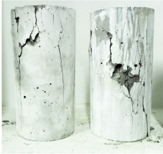
Fig. 4.25 RAC30%: failure modes in tri-axial compression for 4.5 MPa ( left ) and 15 MPa ( right ) confinement levels
