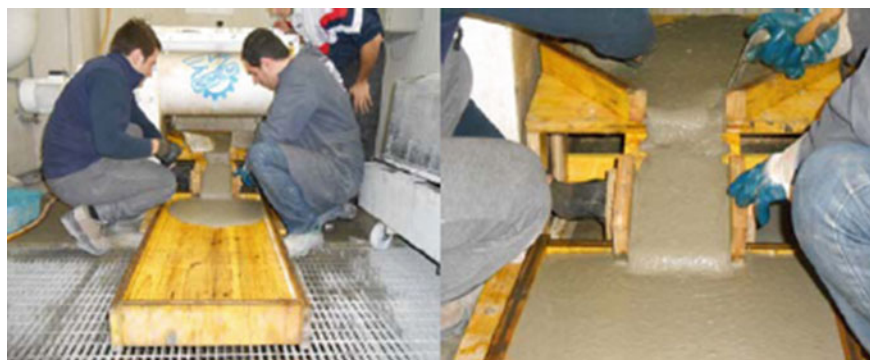
Fig. 9.17 Casting process employed by Ferrara et al. (2015a, b) for self-compacting NFRCC
